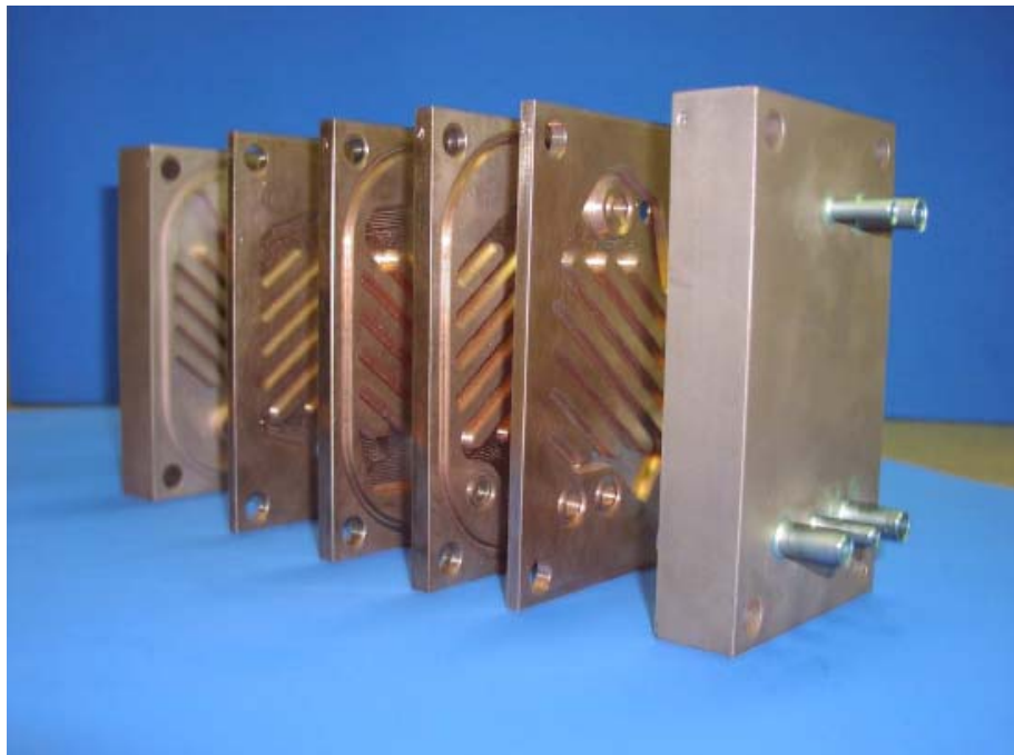
Figure 2: First generation two pass plate-type heat exchanger [1]
